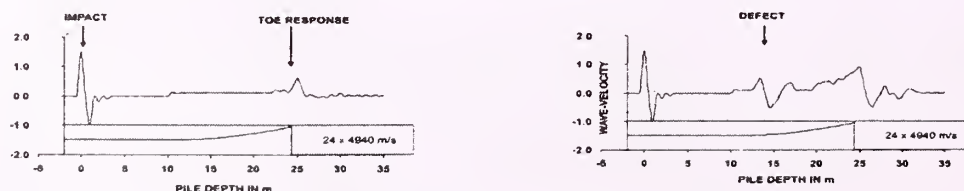
Fig. 1: PIT Velocity versus Depth plot for normal pile (Top) and defective pile (bottom)
