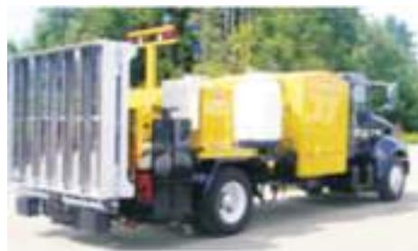
11.3 Infrared road patching technology
