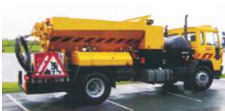
11.2 Velocity Injection Jetpatching Machine
