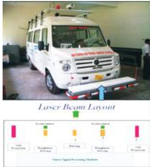
Photo-3 Laser Profilometer Installed in Front of the Survey Vehicle
