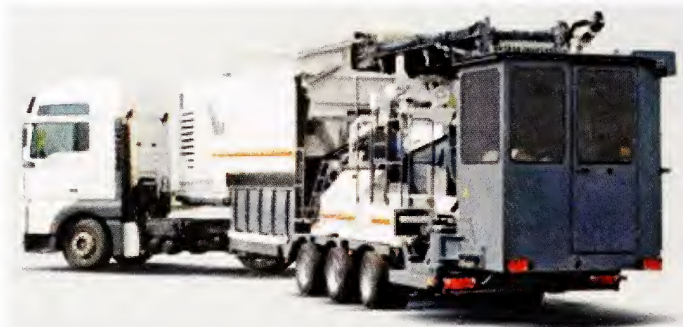
Photo 11.7 Cold Recycling Machine
