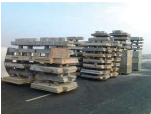
Photo 9 Load Testing by Static Method - a Closeup of Loads
