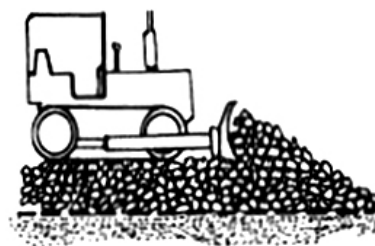
d. SPREAD THE AGGREGATE OVER THE GEOTEXTILE TO THE DESIGN THICKNESS
