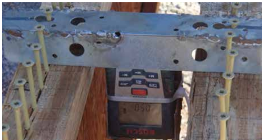
Fig. II-5 Positioning of Laser Distance Measuring Device for Profiling
