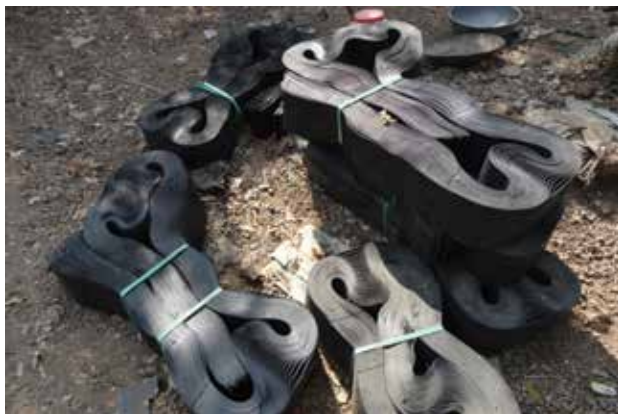
Fig. 6.3a Geocell Panels at Site
