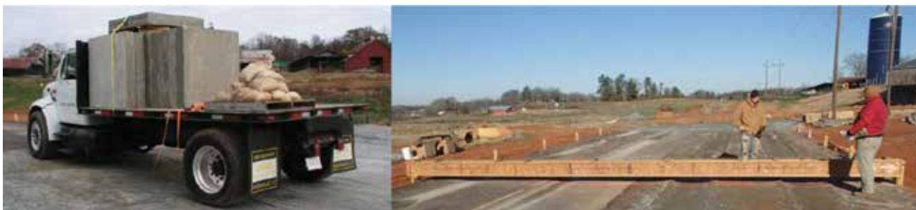
Fig. II-4 Loading Vehicle and Beam for Surface Rut Measurements during Traffic
