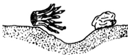
a. PREPARE THE GROUND BY REMOVING STUMPS, BOULDERS, ETC; FILL IN LOW SPOTS
