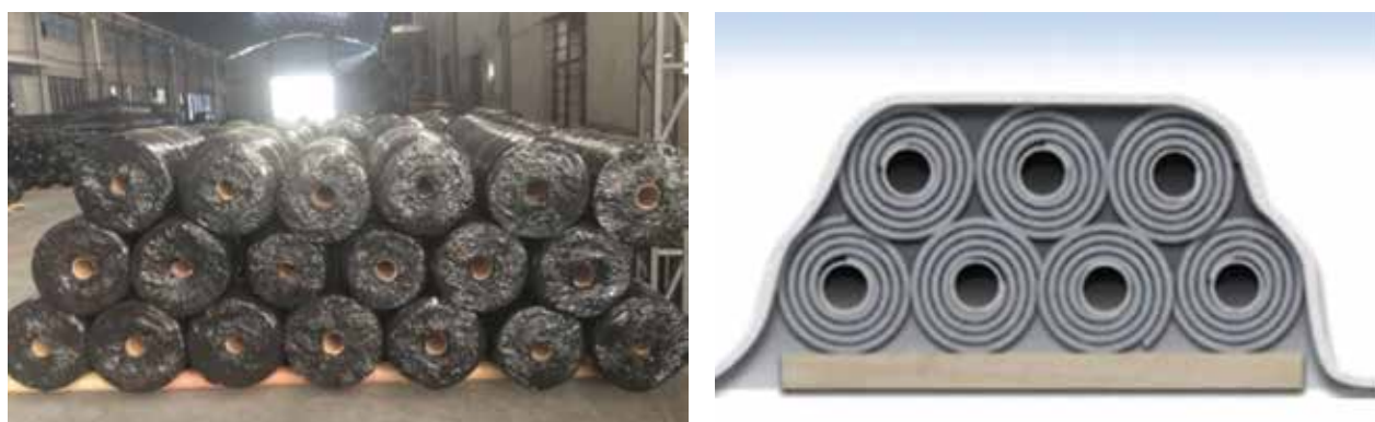
Fig. 6.5 Covering of Geosynthetic Rolls before Use at Site
