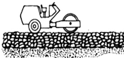
e. COMPACT THE AGGREGATE USING DOZER TRUCK OR SMOOTH DRUM VIBRATORY ROLLER
