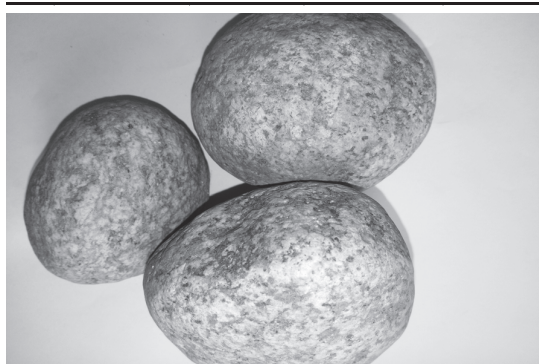
FIG. 7 PARTICLE SHAPE - ROUNDED
