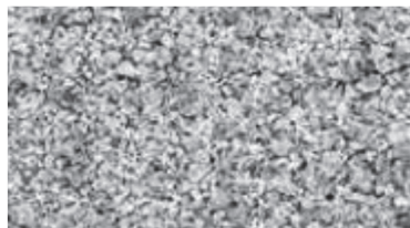
FIG. 2 GRANULATED IRON SLAG AGGREGATE
