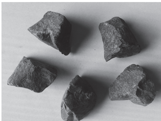
FIG. 9 PARTICLE SHAPE - ANGULAR
