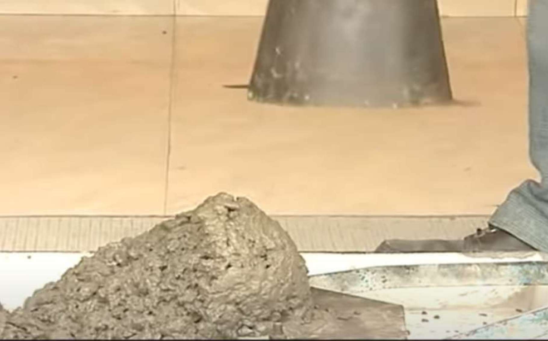
Shear slump - Undesirable
