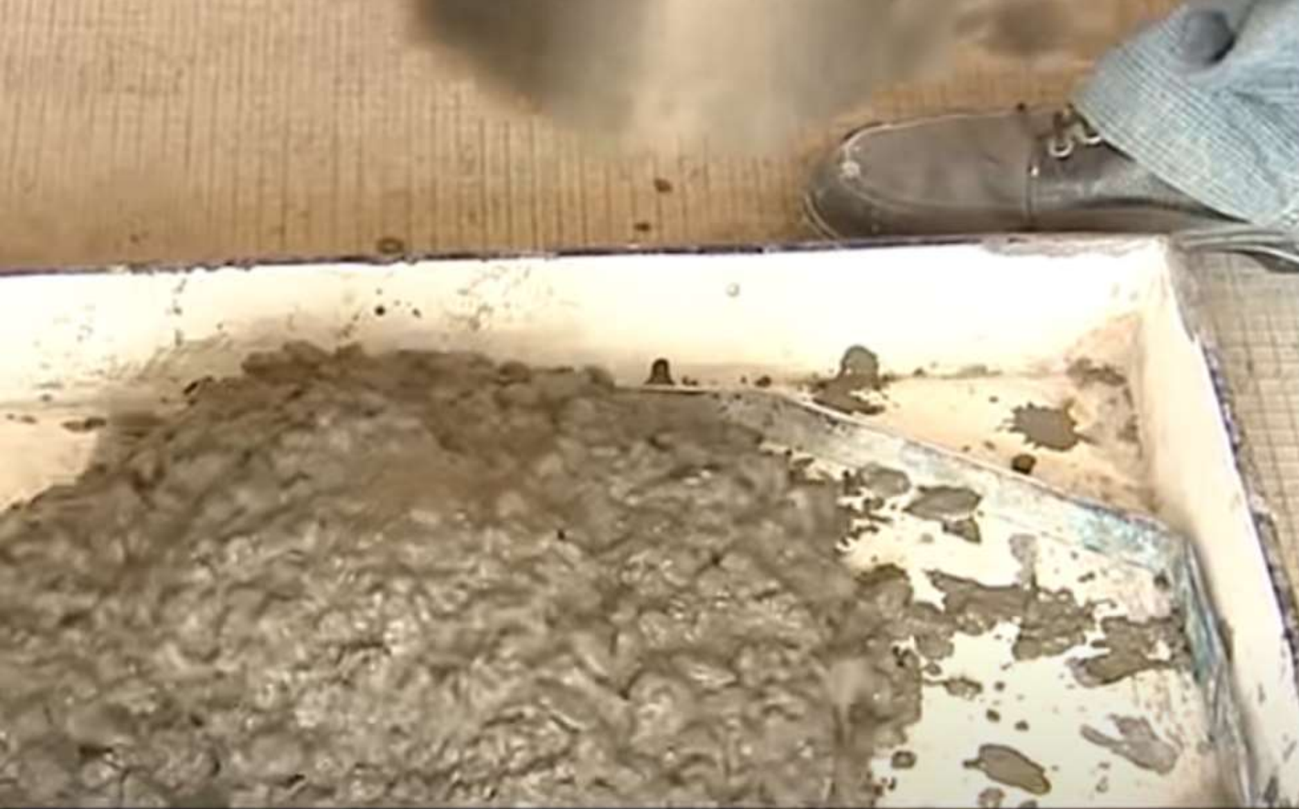
Collapse slump - Undesirable
