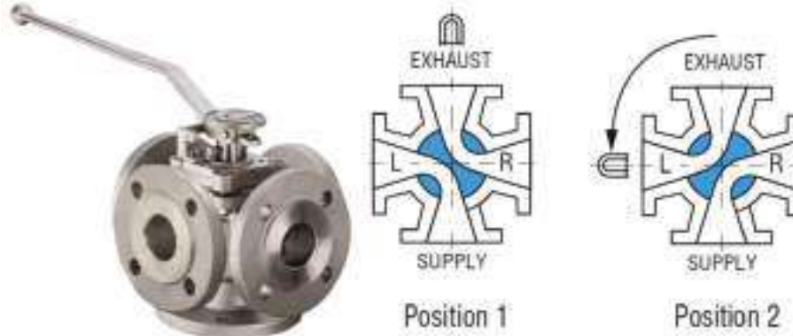
Figure 11.103: Four-way design of Multi-Port Plug Valves
