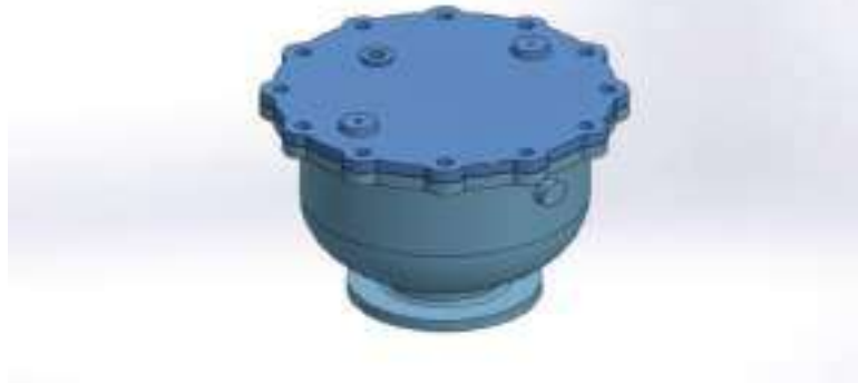
Figure 11.79: Air Release Valves
