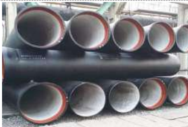
Figure 11.6: Polyurethane coated pipe
