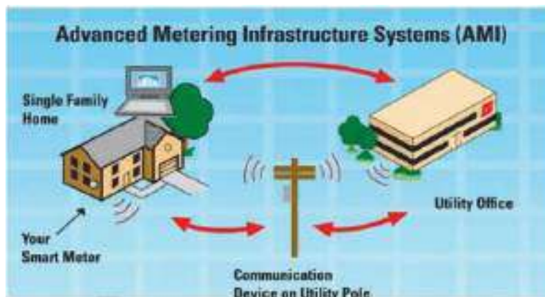
Figure 13.15: Advanced Metering Interface (AMI)
