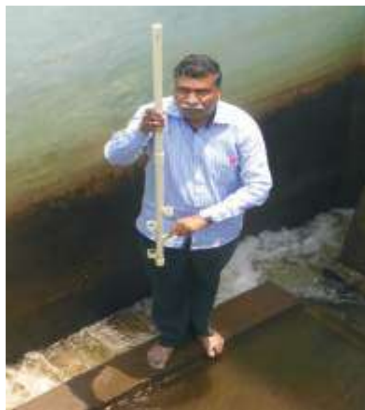
Figure 8.39: Checking Media Expansion During Backwash using Sand Expansion Stick
