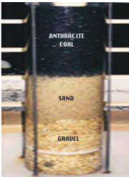
Figure 8.38: Pilot Plant for Dual Media Filters
