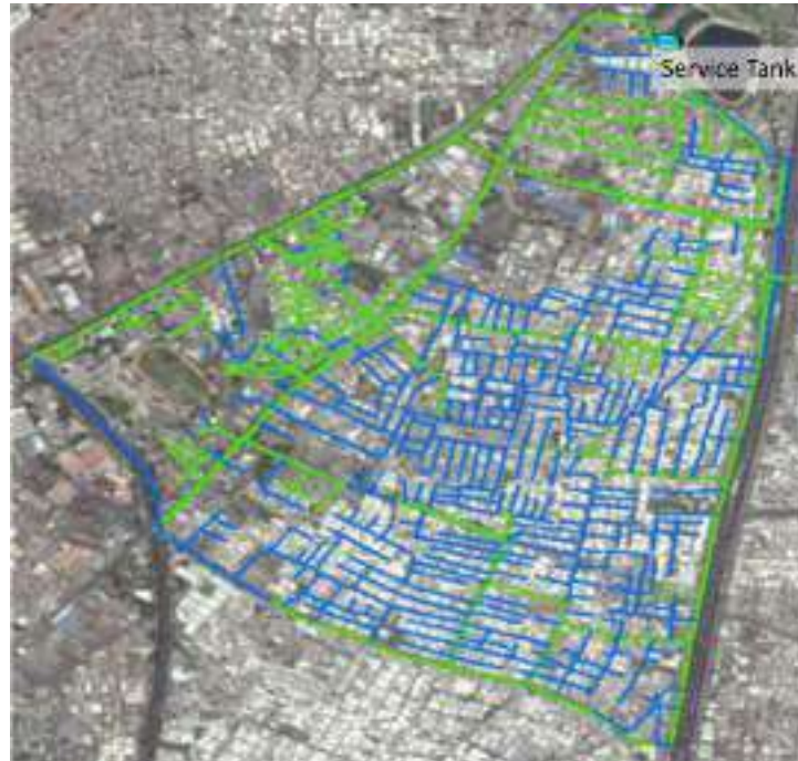
Figure 1: Operational zone of 'Sajipur Old' in Ahmedabad (existing pipes in green and new pipes in blue colour)
