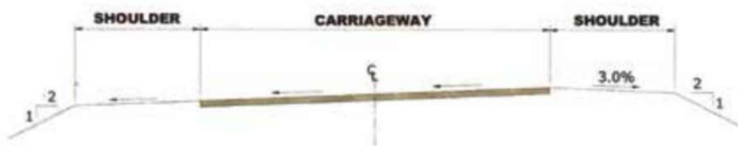
Fig. 10.1. Typical One-way Camber in Super Elevated Sections
