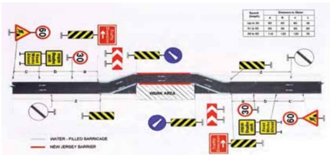
Fig. 7.18 Upgrading of 1 L / Intermediate Lane to Two Lane with Shoulders
