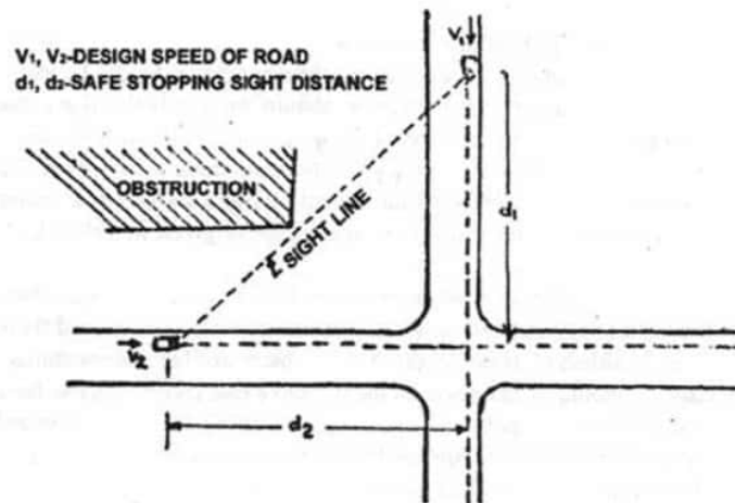
Fig 7.1 (a) Minimum sight triangle at uncontrolled intersections
