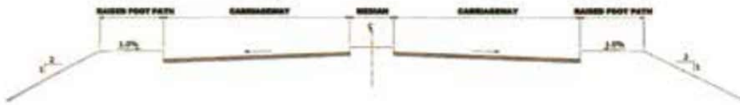
Fig. 10.3. Typical Cross Section of divided carriageway with kerbs (Urban situation)
