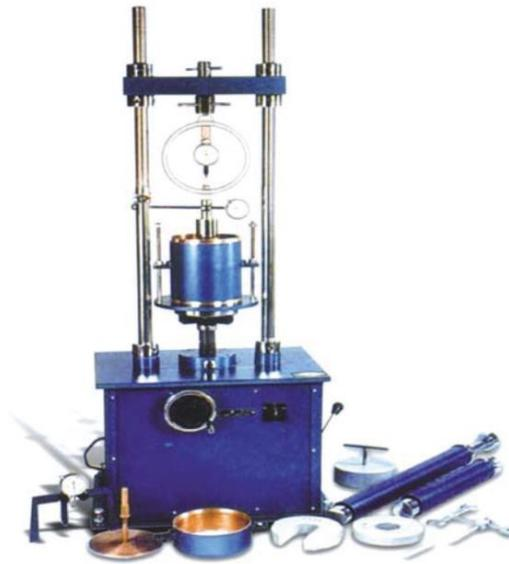
LABORATORY CBR TEST APPARATUS
