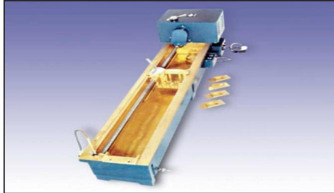
**Ductility Test Apparatus**
