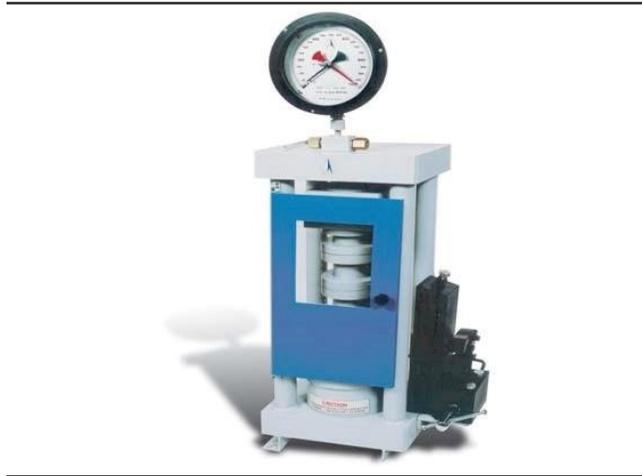
**HAND OPERATED COMPRESSION TESTING MACHINE**
