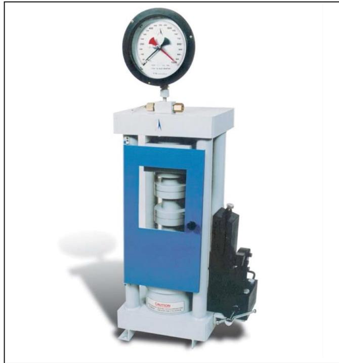
**HAND OPERATED COMPRESSION TESTING MACHINE**
