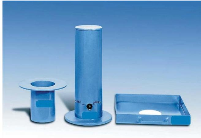
**SAND POURING CYLINDER APPARATUS**
