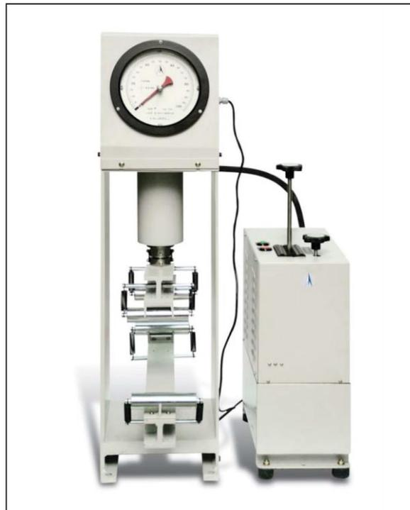
FLEXURE TEST APPARATUS
