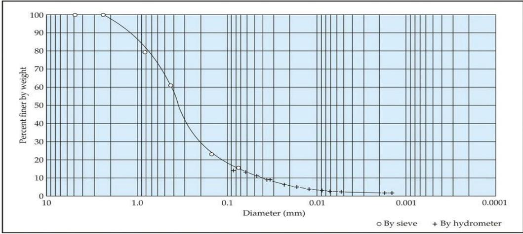
Figure 1 Typical Grain Size Distribution Diagram
