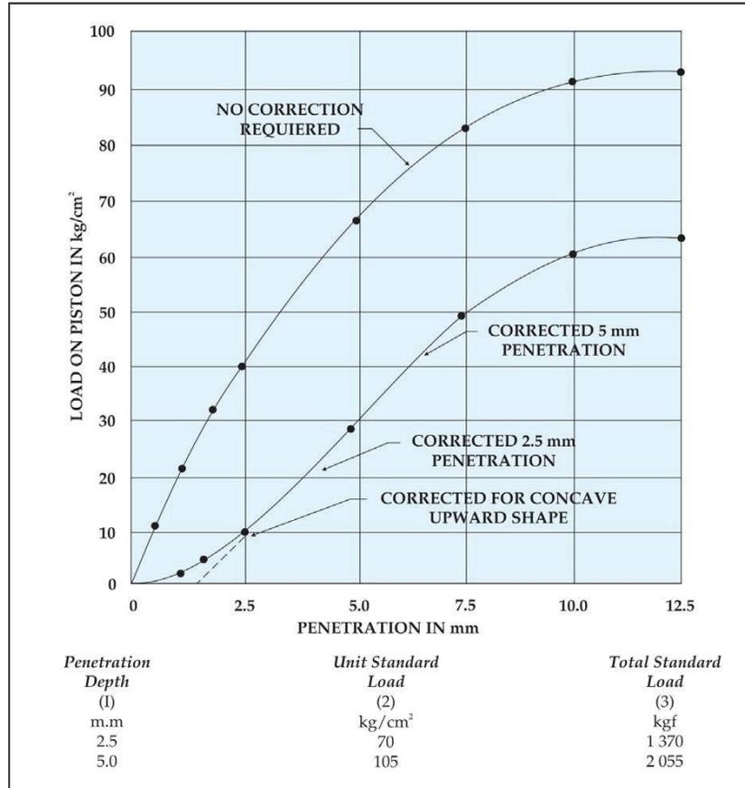
Figure 6 Correlation of Load Penetration Curves
