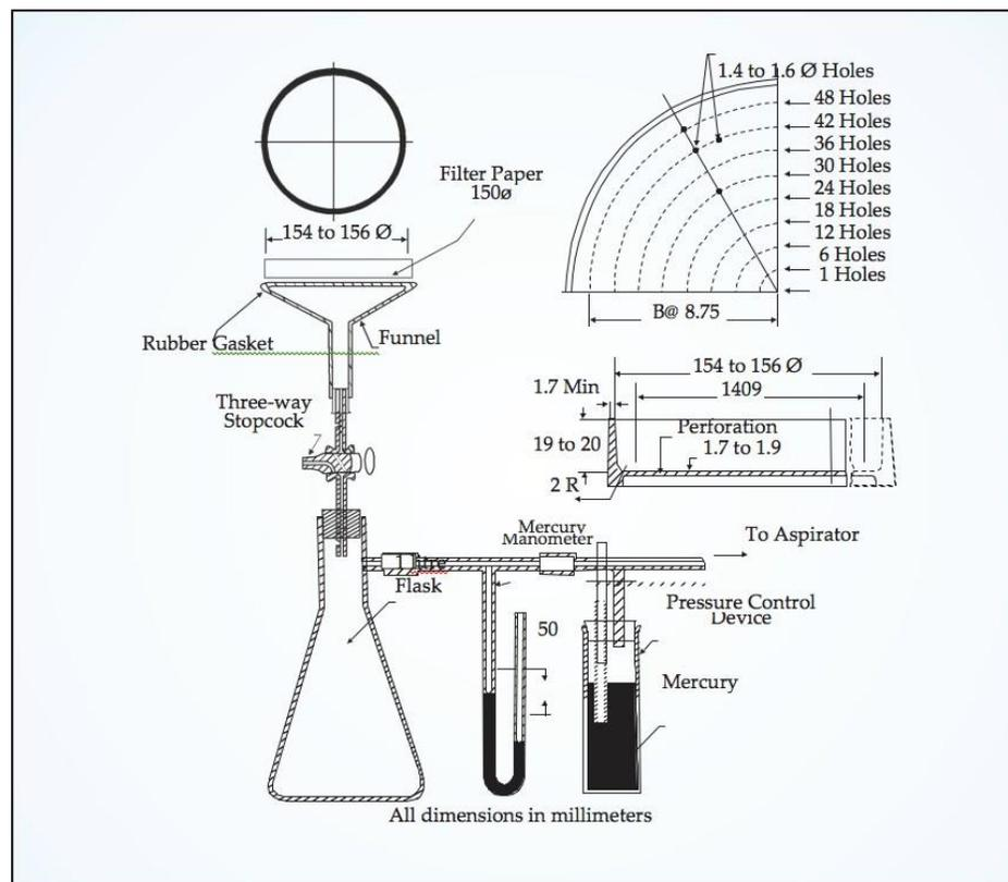
FIG 8 APPARATUS ASSEMBLY FOR WATER RETENTION TEST
