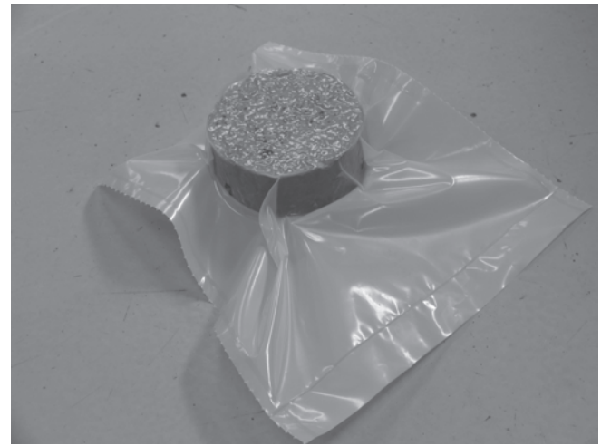
Figure 4.10 Asphalt Mix Sample in Sealed Bag
