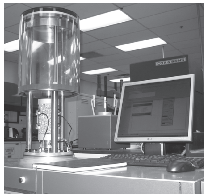
FIGURE 10.6 AMPT (Environmental Chamber Raised, Instrumented Specimen Loaded)
