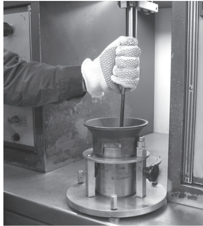
FIGURE 8.10 Rodding Mix in Mold
