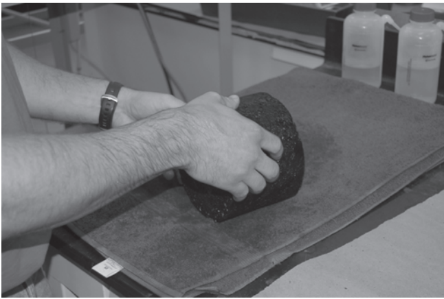
Figure 4.8 Determination of SSD mass of specimen
