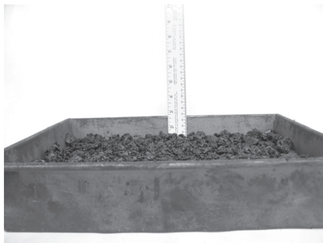
FIGURE 4.6 Mixture conditioning for volumetric mix design
