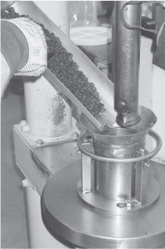
FIGURE 8.7 Mechanical Kneading Compactor for the Preparation of Hveem Test Specimens
