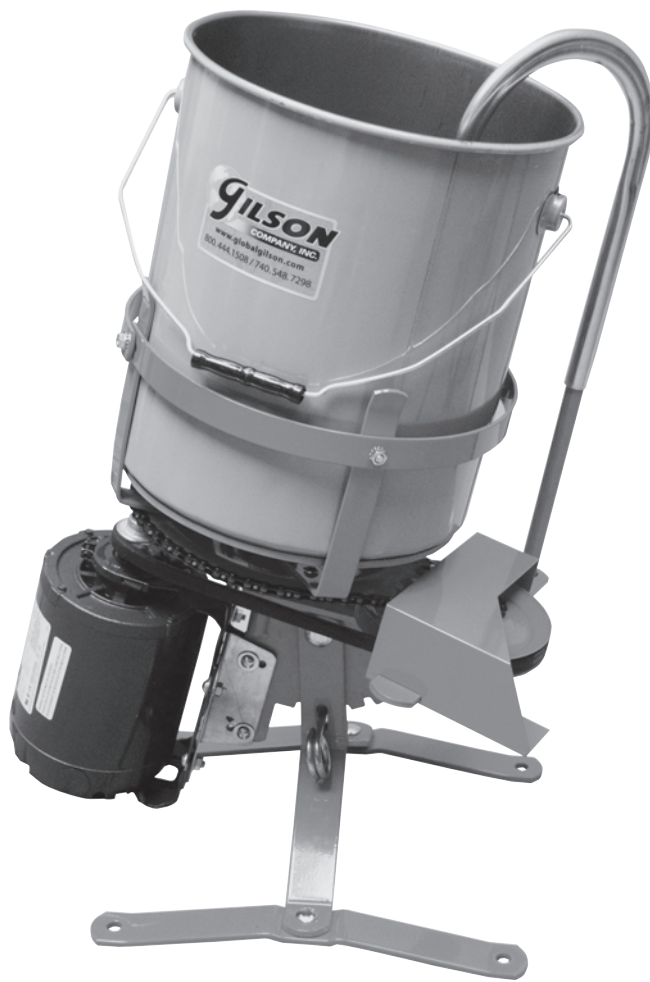
FIGURE 4.3 Five-gallon bucket mixer
