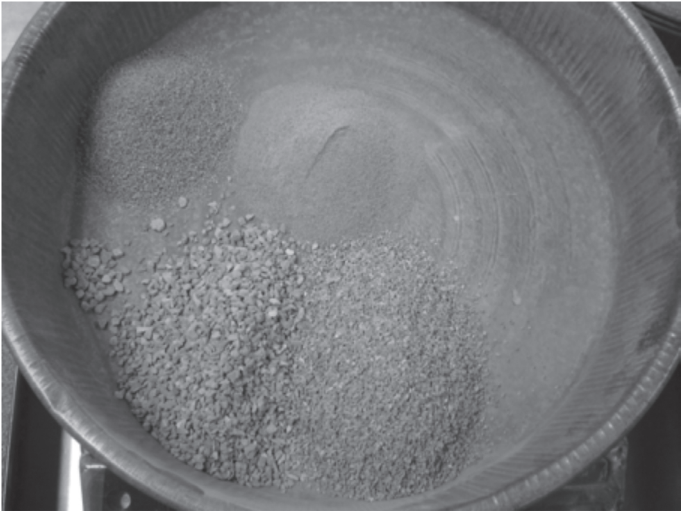
FIGURE 3.10 Batching into distinct piles
