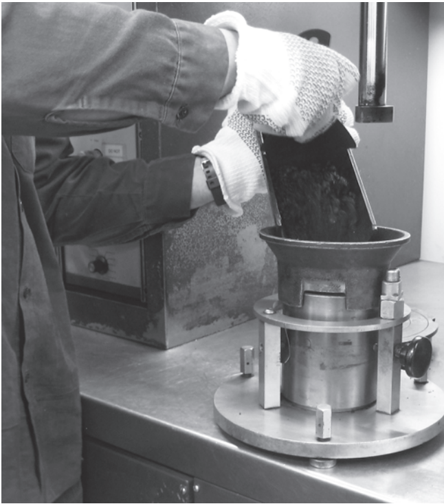
FIGURE 8.9 Transfer of Mix to Mold
