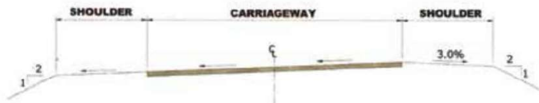
Fig. 10.1. Typical One-way Camber in Super Elevated Sections
