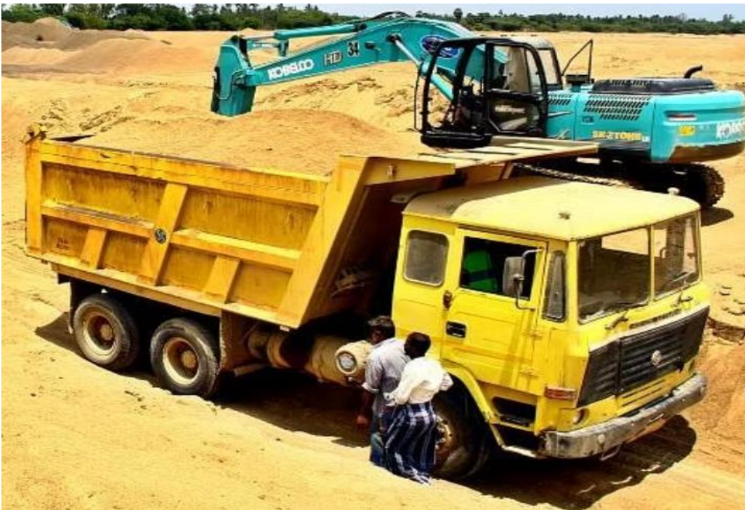
Fig: HCVs with Rear Two Axles with Dual Tyres and Front Single Axle with Single tyre
