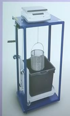
Fig. 2: Setup of Water Absorption Test
