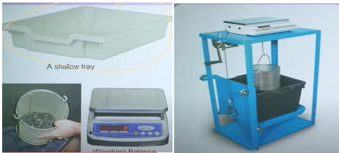
Fig. 2: Setup of Water Absorption Test
