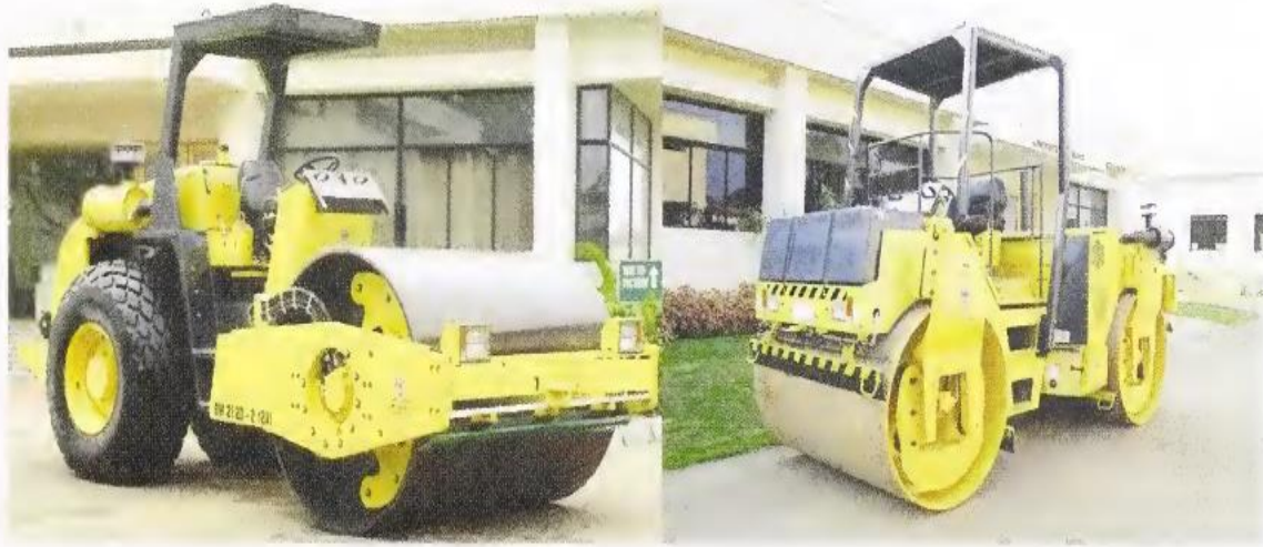
Fig. 6. Smooth Drum Vibratory Roller
