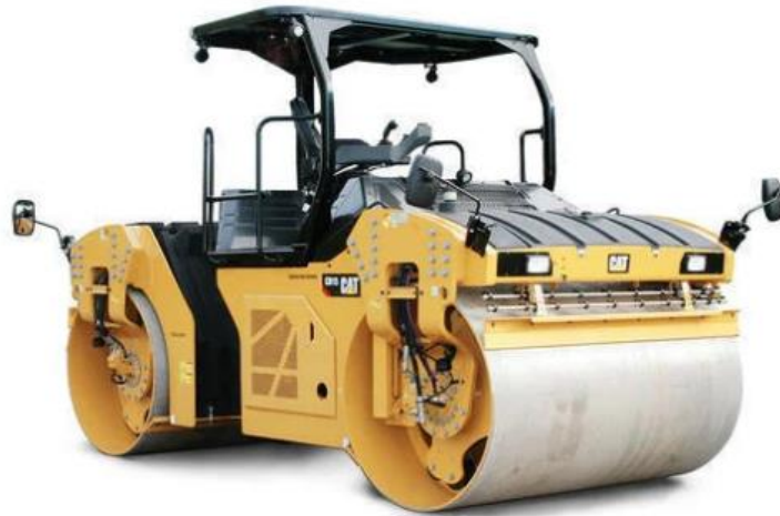
Fig.8. Tandem Vibratory Roller
