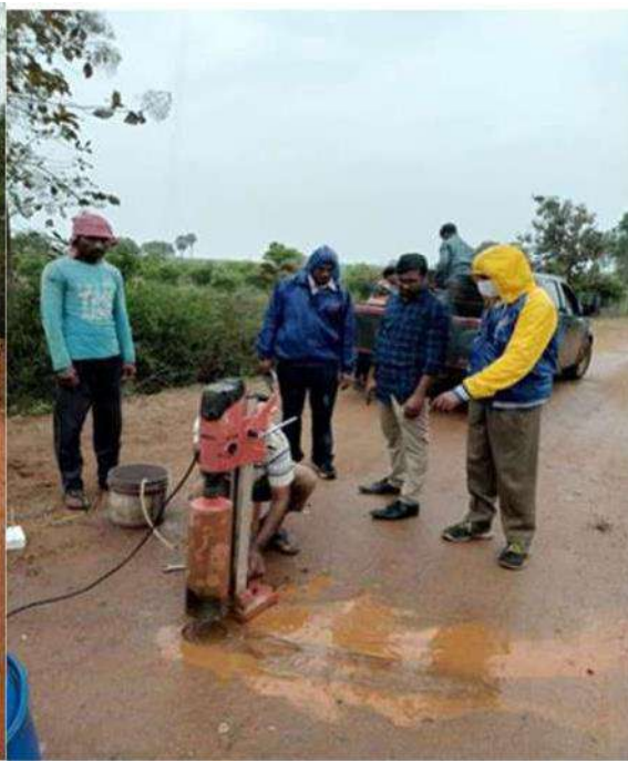
Extraction of Cores for testing UCS
