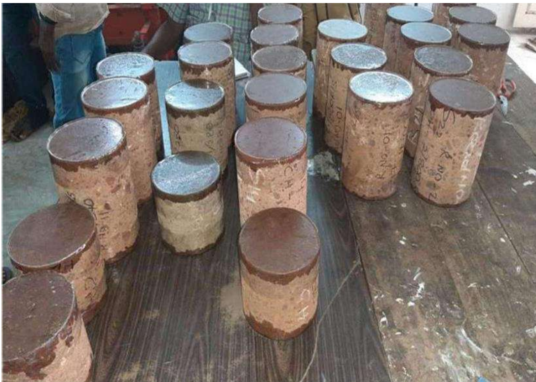
Cores Extracted from Stabilized Base and ready for testing.
